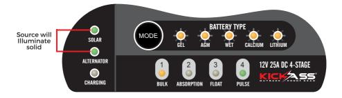
IMPORTANT : You must select 'LITHIUM' as the battery type by using the 'MODE' button prior to connecting it to a lithium battery in sleep mode to attempt recovery.
